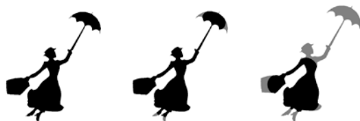
Fig.4 Consecutive contact configuration of a flat-ended stamp in form of "Marry Poppins" calculated with adhesive BEM [20].
